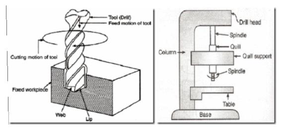
Working Principle of Drill machine Sensitive Drill Machine/Drill Press
