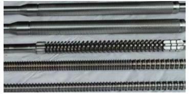
Broaching relies on a toothed tool called a broach. One of the most essential traits of a broach is the rise per tooth, which indicates the amount of material each tooth removes every pass. These teeth are then broken down into sections along the body of the tool: the roughing, semi-finishing and finishing sections.
