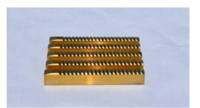
Broaching is a machining process that uses a toothed tool to remove material in a consistent and accurate way. There are two types of broaching services, linear and rotary, which are used to produce different kinds of machining finishes, but in either case, <u>production broaching</u> is typically only used for precision applications and high-quantity production.
